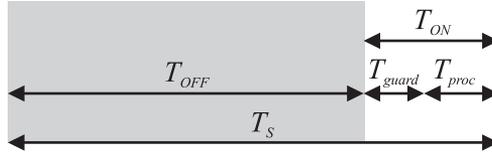
Fig 3 – The complete time synchronization period.
