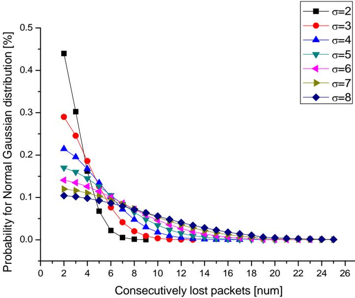
**Fig. 5** – Probability of consecutively lost packets for Normal Gaussian distribution for different  $\sigma$  as parameter.
