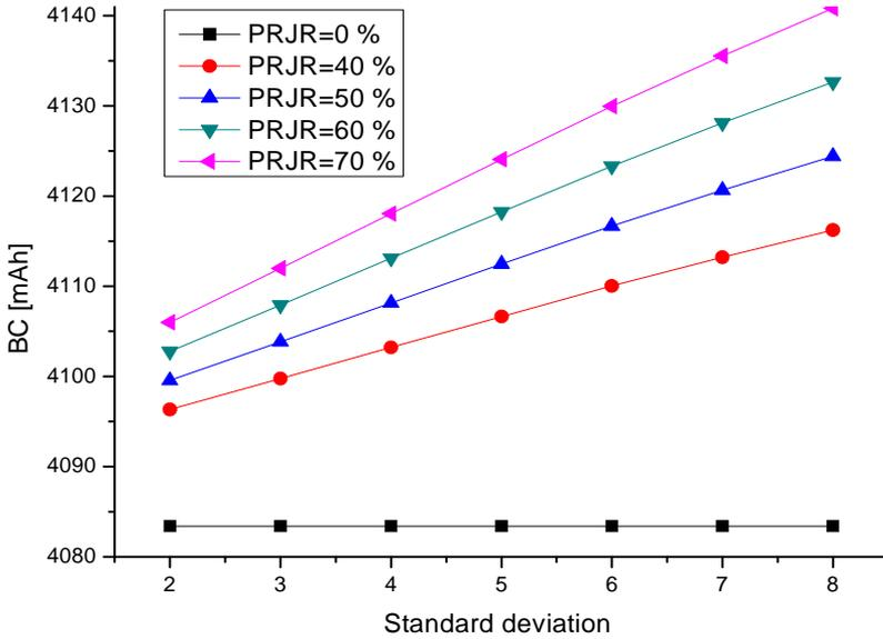
**Fig. 6** – Battery capacity for different PRJRs for single year SN's working period and  $T_{\Sigma} = 1$  s.
