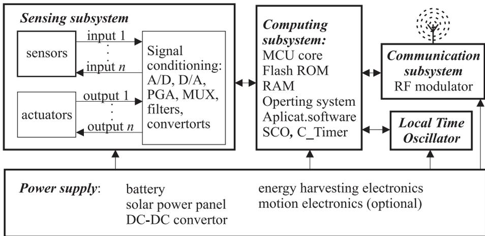
Fig. 1 – System architecture of a typical sensor node.
