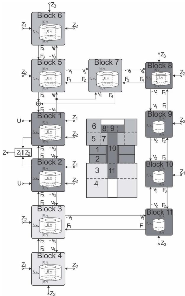
**Fig. 1** – Block diagram of the ultrasonic transducer model.
