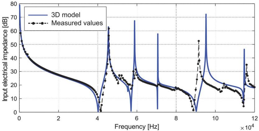
**Fig. 5** – Simulated and experimental input electrical impedance versus frequency for the Transducer2.
