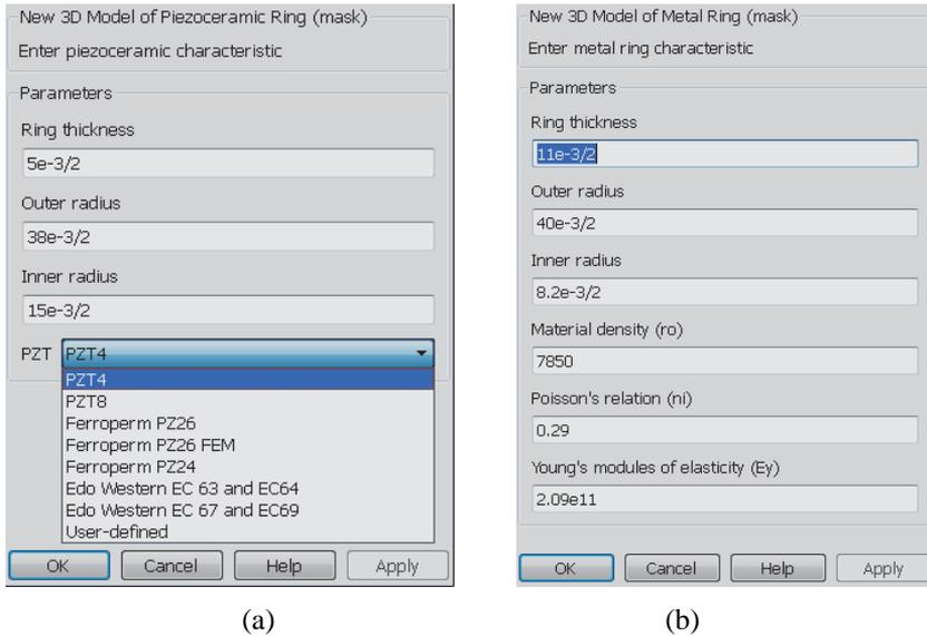
**Fig. 3** – Interface for insertion of piezoceramic parameters (a) and metal ending parameters (b).
