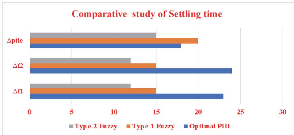
Fig. 5 – Comparative study of settling time for different control techniques.
