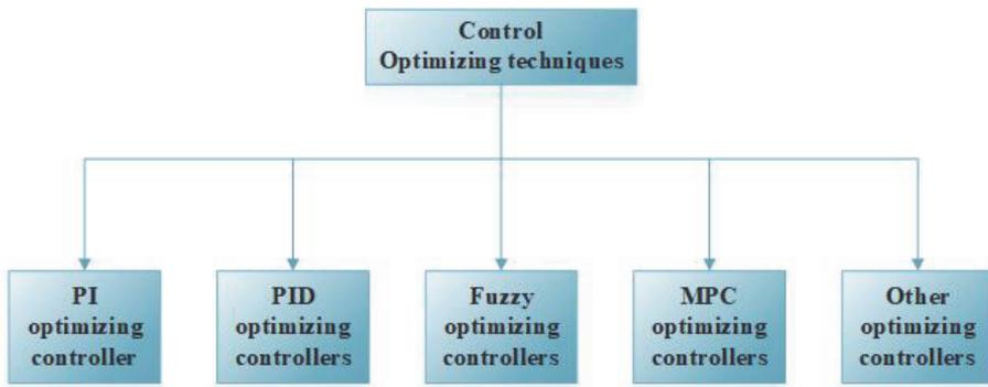
Fig. 1 – Classification of different control optimizing techniques.
