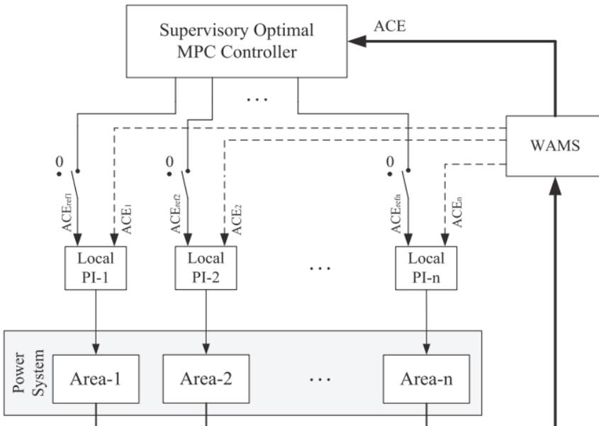
**Fig. 3** – Two-level Supervisory MPC control technique for n-area power system.
