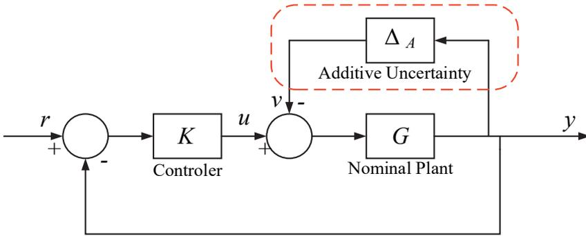
Fig. 2 – Feedback system with inverse additive perturbation.
