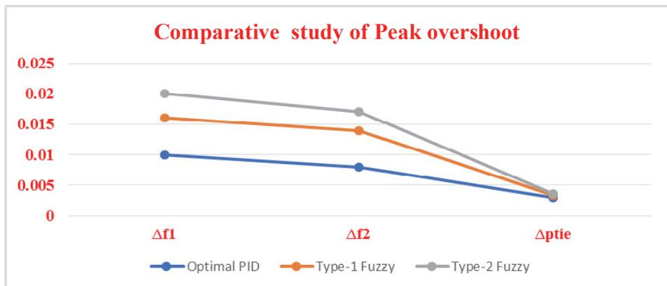
Fig. 6 – Comparative study of peak overshoot for different control techniques.
