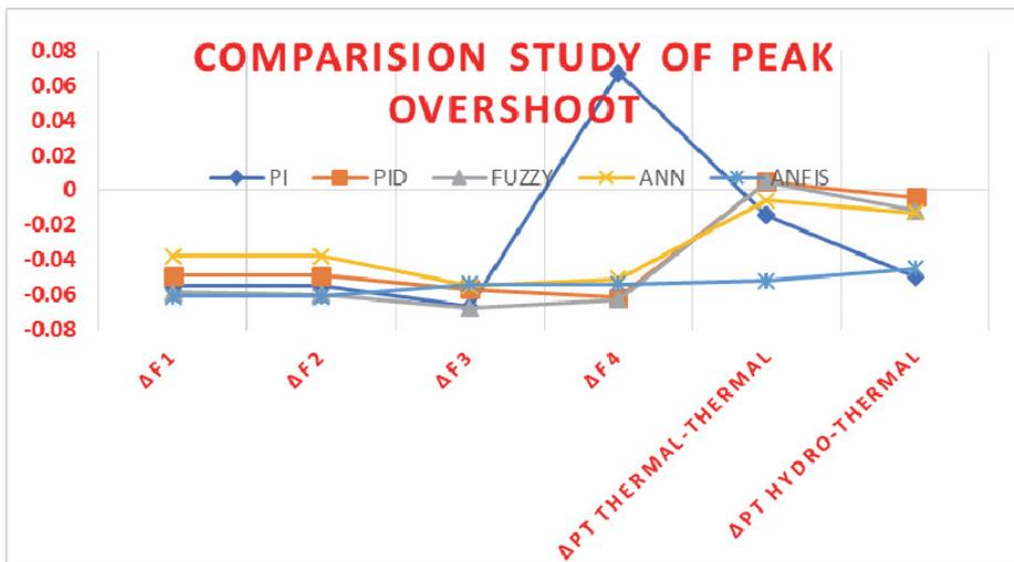
Fig. 8 – Comparative study of peak overshoot for different control techniques.
