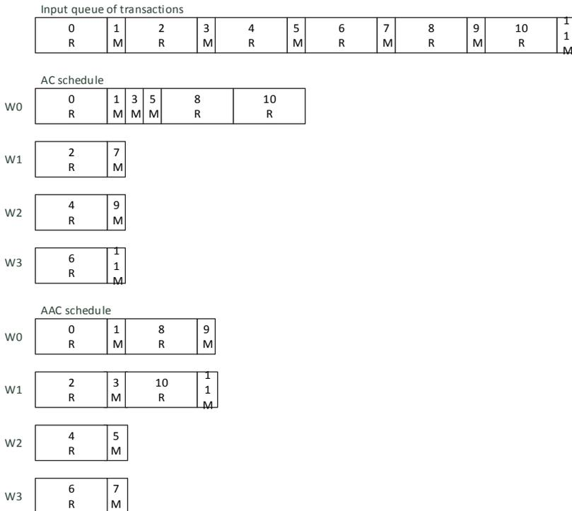
**Fig. 3** – Transaction schedules for AC and AAC algorithms, for RDW workload and four workers.
