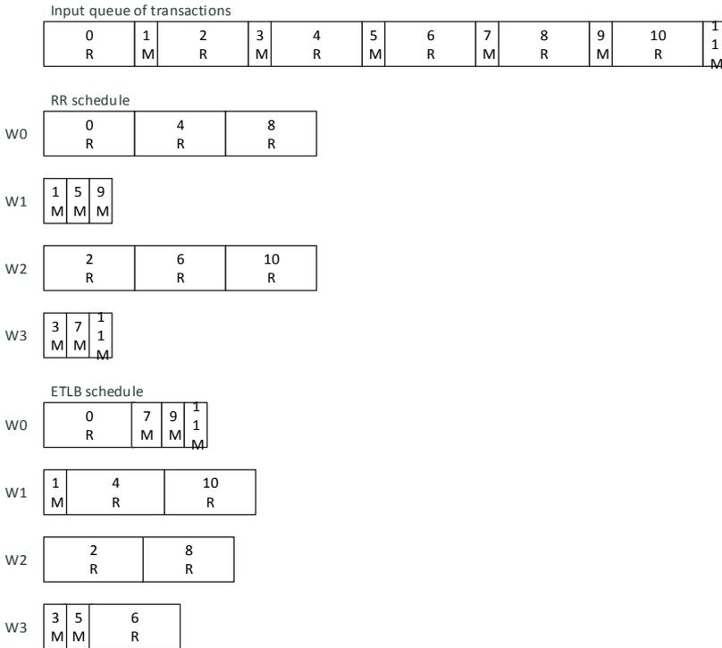
**Fig. 2** – Transaction schedules for RR and ETLB algorithms, for RDW workload and four workers.
