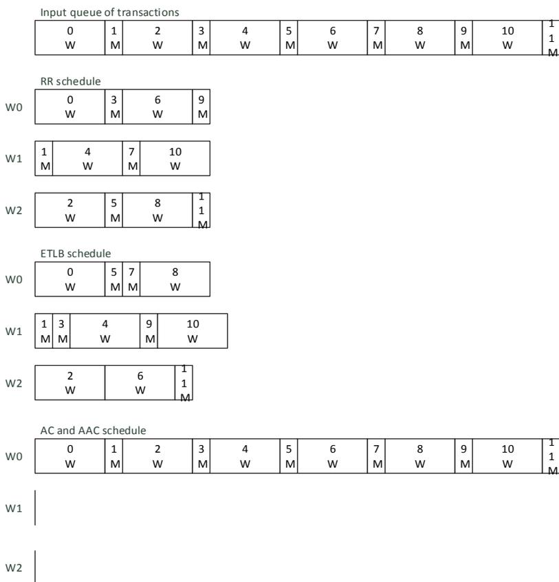
**Fig. 5** – Transaction schedules for all the algorithms, for WDW workload and three workers.
