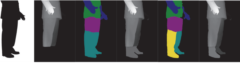
Fig. 6 – Left to right: (1) input image (censored); (2) depth map from AgiSoft MetaShape; (3) segmentation map from WSHP neural network; (4) output of the proposed method for (3); (5) manually corrected segmentation mask; (6) output of the proposed method for (5).
