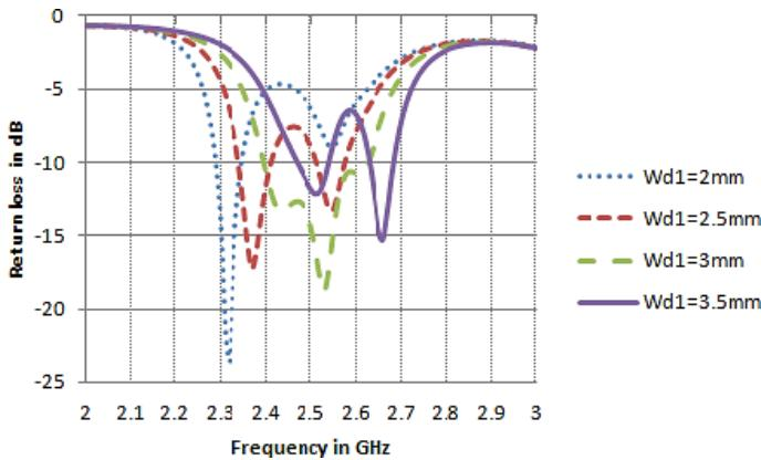
**Fig. 5 – Return loss variation when width  $W_{d1}$  is changed.**
