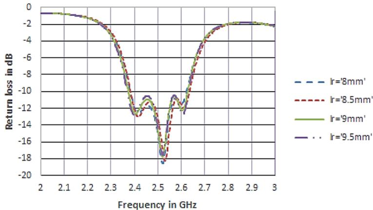
**Fig. 11** – Return loss variation when width  $l_r$  is changed.
