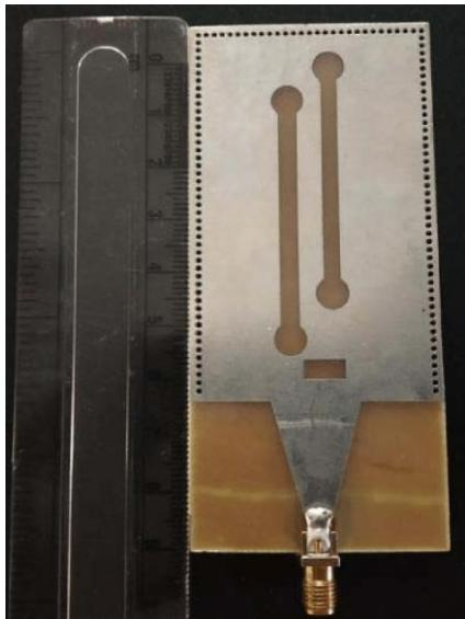
**Fig. 12 – Photograph of the fabricated antenna.**
