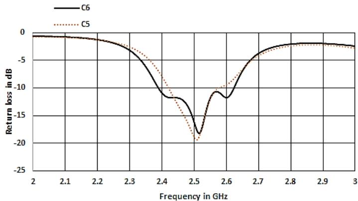
**Fig. 9** – Return loss variation for configurations C5 and C6.
