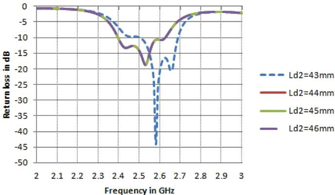
Fig. 8 – Return loss variation when width  $L_{d2}$  is changed.
