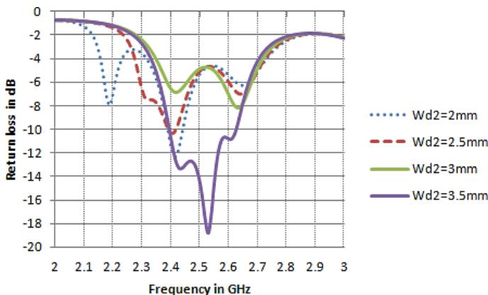
**Fig. 6 – Return loss variation when width  $W_{d2}$  is changed.**
