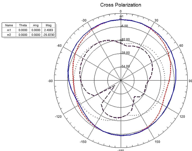
**Fig. 15 – Radiation pattern with cross-polarization.**
