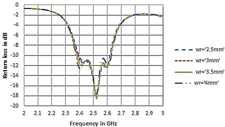
**Fig. 10** – Return loss variation when width  $w_r$  is changed.
