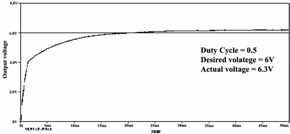
Fig. 22 – Open Loop Buck Converter Output using SET.
