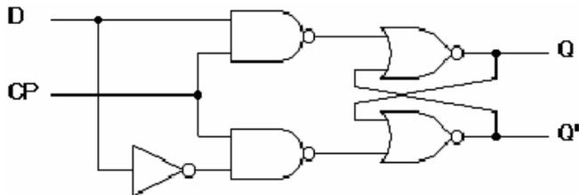
Fig. 14a –D Flip Flop.
