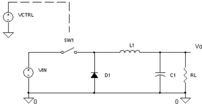
**Fig. 16 – Buck Converter.**
