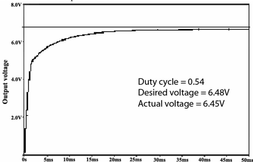
Fig. 24. – Closed Loop Buck Converter Output using SET
