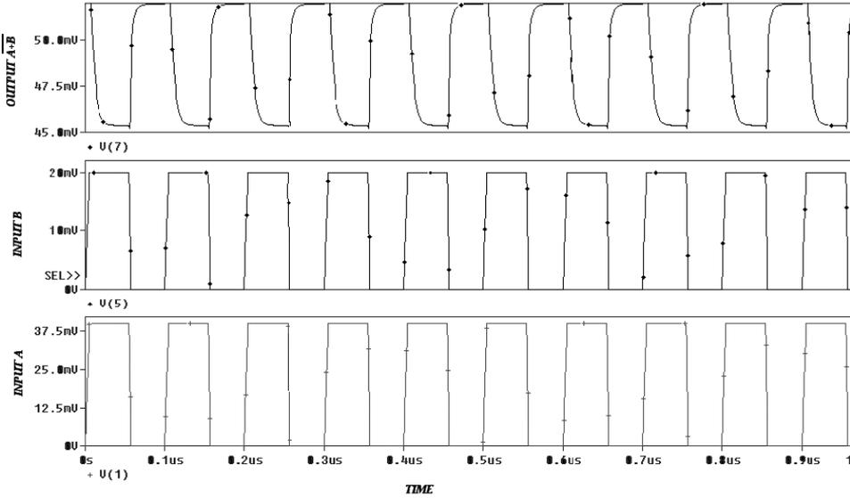
Fig. 7 – NOR Gate input and Output Response.
