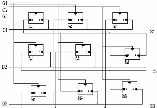
Fig. 17 – 3 Bit Shift Register.
