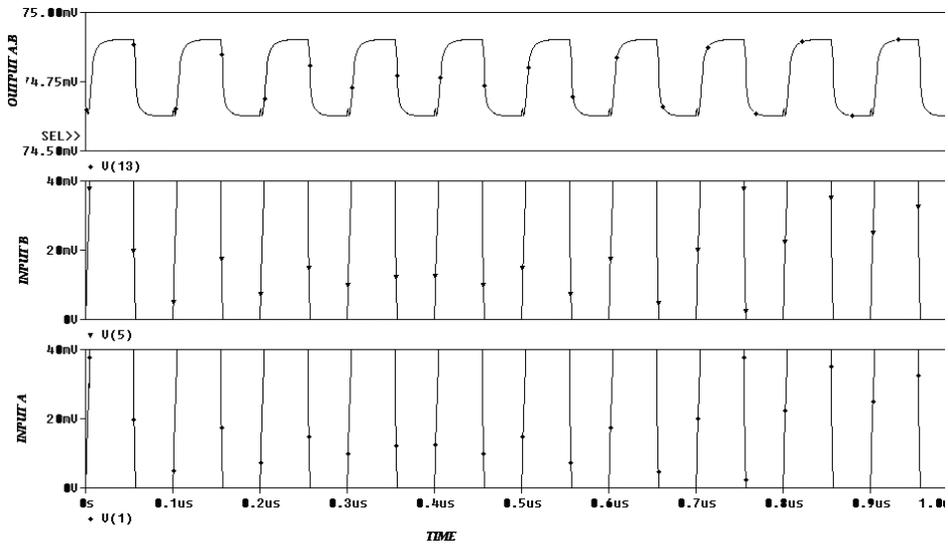
Fig. 12 – AND Gate input and output Response.
