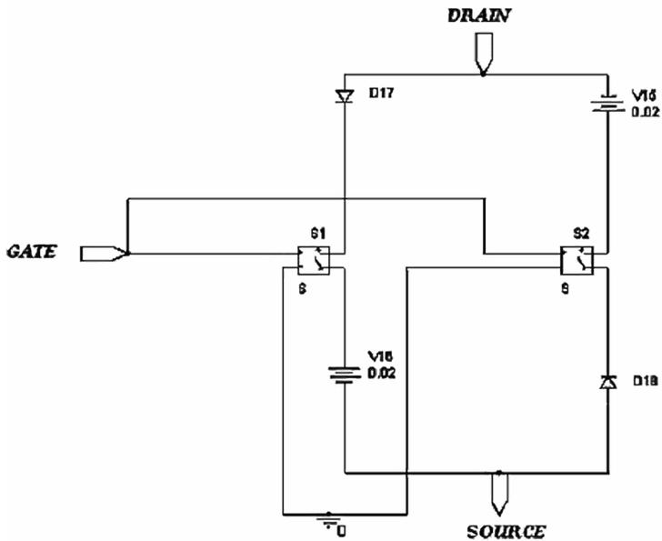
Fig. 2 – SET Equivalent Circuit-Model.
