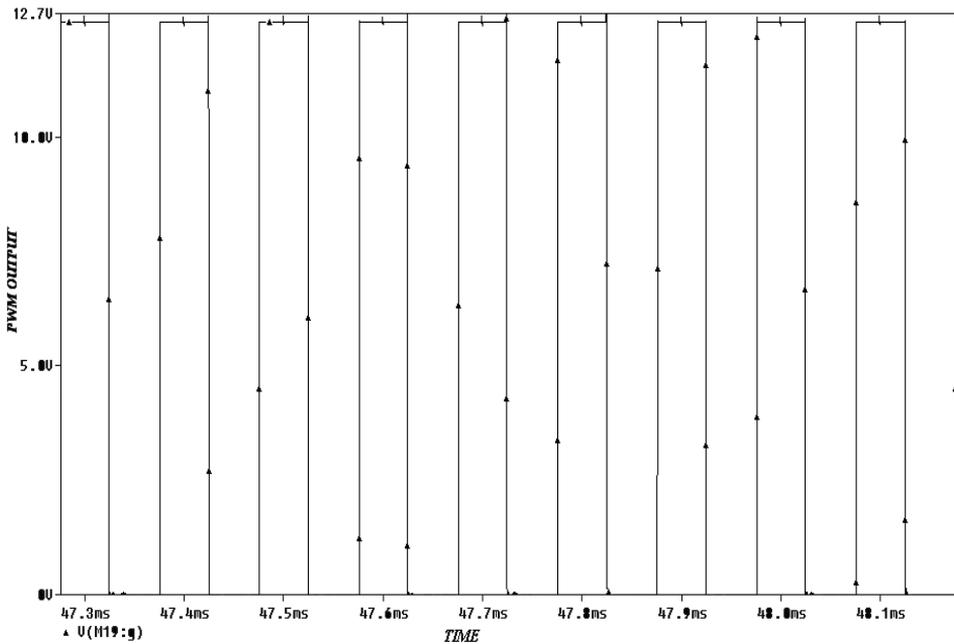
Fig. 23 – Closed loop PWM output.
