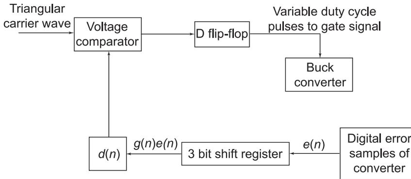
Fig. 15 – Control Circuit of PWM Controller.
