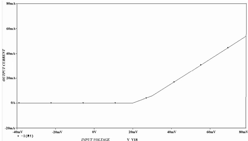
Fig. 3 – SET I-V characteristics–Model 3.
