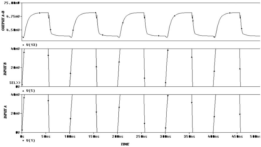
Fig. 13 – OR Gate input and output Response.
