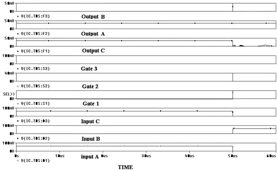
Fig. 18 – 3 Bit Shift Register Output.
