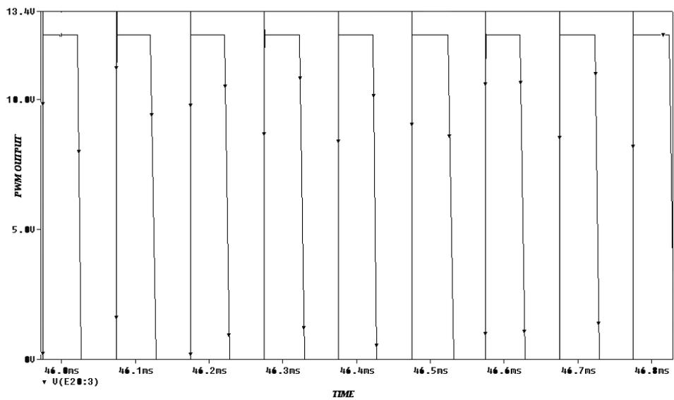
Fig. 21 – Open Loop PWM Output using SET.
