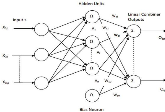
Fig. 2 – Radial Basis Function Network model.
