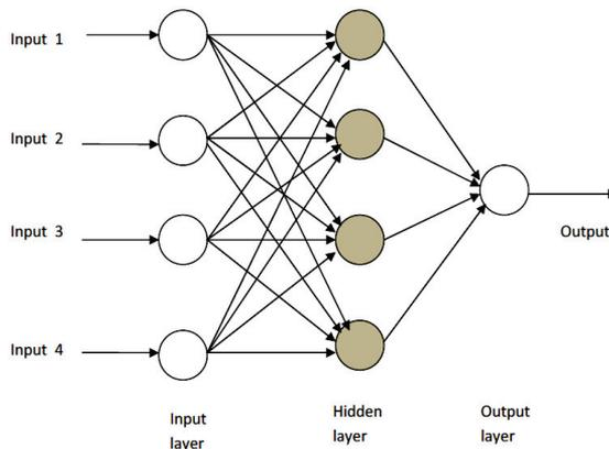
Fig. 1 – Topology of a three layered MLP.
