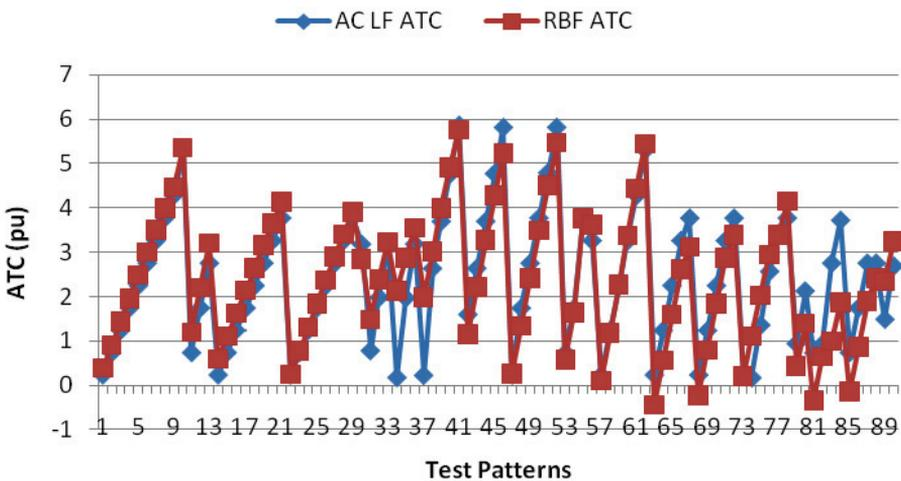
Fig. 7 – 75-bus practical system comparison of RBF ATC and AC LF based ATC.
