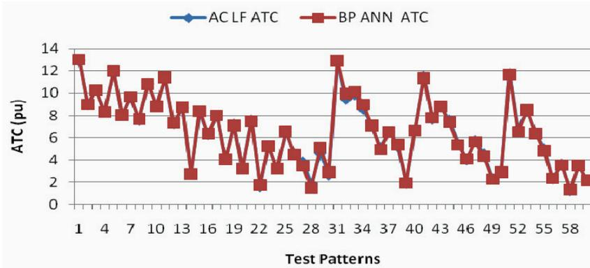
**Fig. 4** – IEEE 24-bus RTS comparison of BPA Neural Network ATC and AC L F based ATC.
