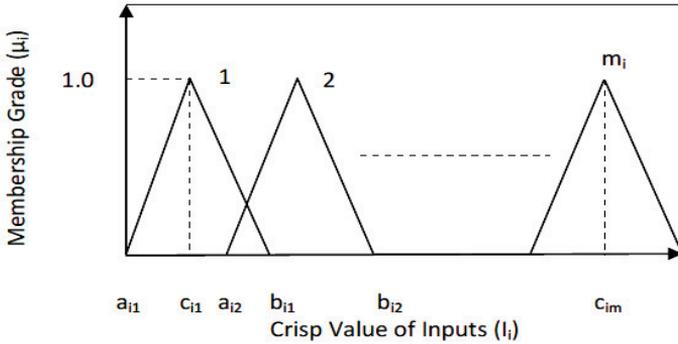
Fig. 3 – Triangular membership function for  $i^{\text{th}}$  input.
